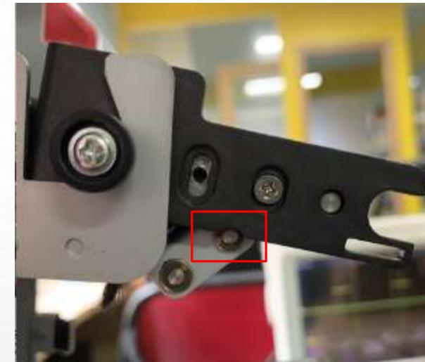
**Note:** The deformation of the Ribbon Led bracket is caused by the artificially misplacing of the ribbon to the bottom of the print head and then press the top cover.
