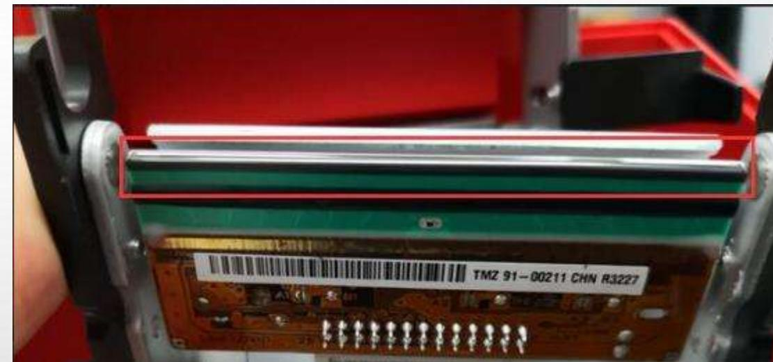
**Cause 2:** The print head signal line damage or poor contact
