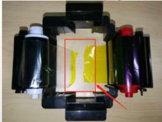
**Solution:** Remove the ribbon, tape the break with tape, then roll the broken ribbon to the white end
