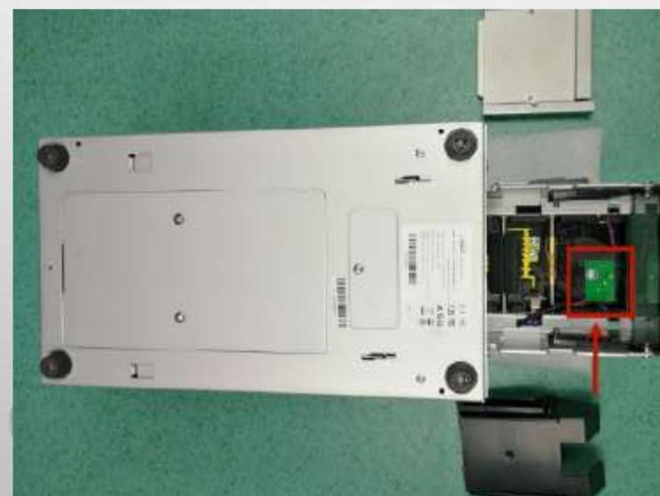
**Solution:** Replace the ADF sensor
