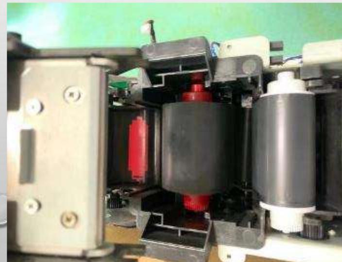
**Cause 5: Dirt in the cam sensor**
