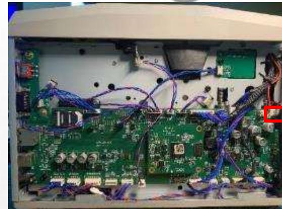
**Solution:** If the print head cable is not broken, please re-plug the cable
