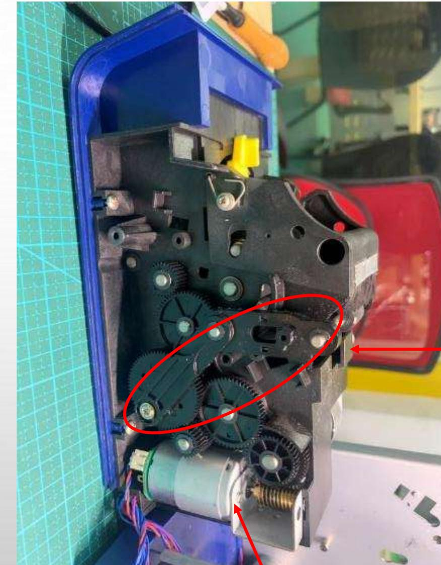
ADF card feed motor (reverse card feed cam)
