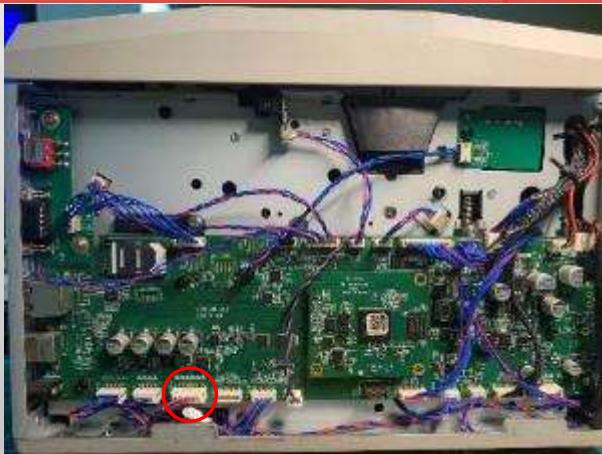
**Solution:** The motor does not rotate during the boot self-test, please check whether the wiring is normal, if no problem with the wiring, replace the CAM motor
