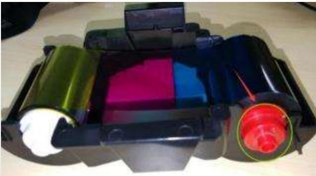
**Solution:** Replace the ribbon and test, confirm whether or not the ribbon chip problem is, replace the ribbon if it was.
