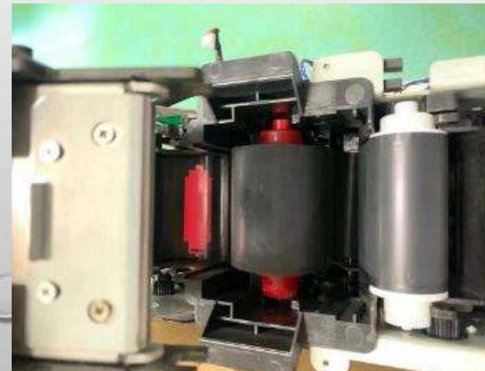
**Cause 5:** Poor contact with the core board, resulting in gear jams
