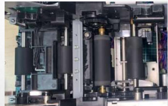
**Note:** Severe messy pattern is usually caused by improper adjustment of clamping plate artificially. If the clamping plate has not been moved, then there are some substances dropped into the ribbon drive gear or TPH cam gear, which causes the gear to rotate abnormally.
