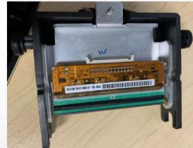
**Note:** Print head bracket breakage is usually caused by the ribbon up shrapnel failure so that the ribbon collapse, when the top cover closed, the print head would be crushed due to ribbon resistance deviated from the guide slot on both sides of the print head
