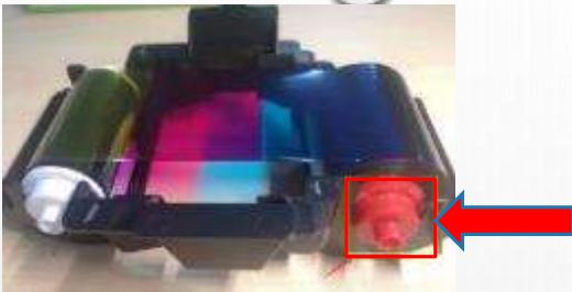
**Cause 2:** RF coil induction instability, the counting of the ribbon chip fails to be deducted
