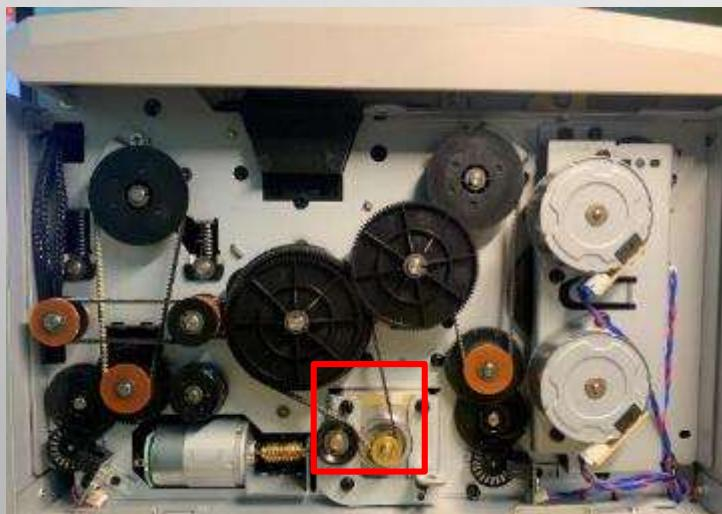
**Solution:** Check if the belt is broken, check if there is any other substances jammed between the gears
