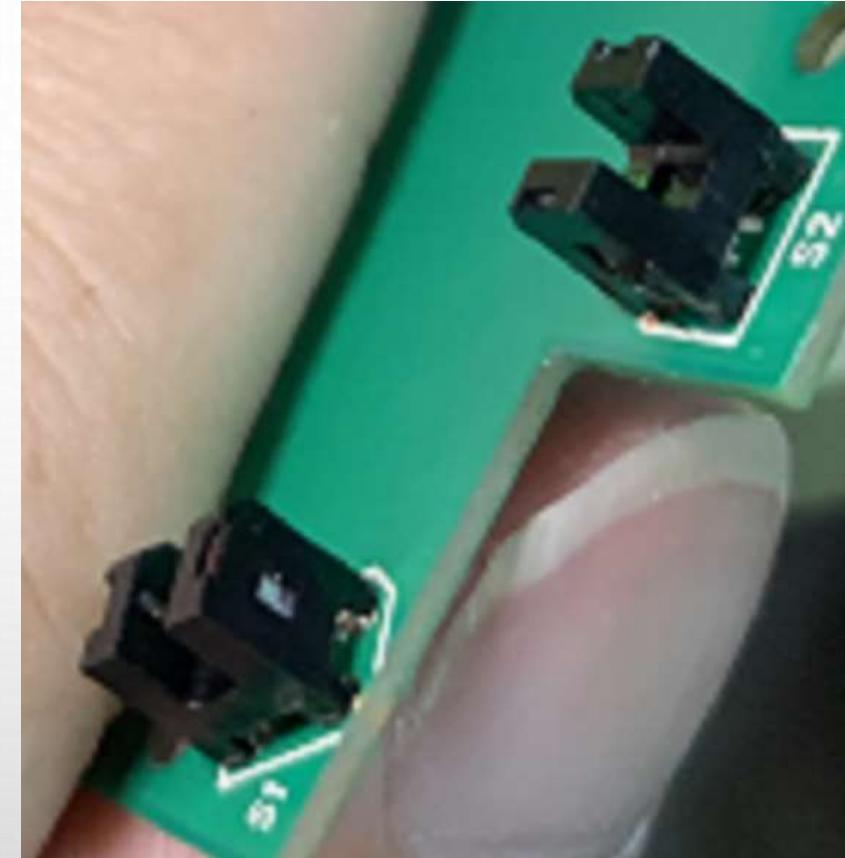
**Note:** Dirt in the cam sensor will cause the sensor to misjudge the position of the cam mechanism, resulting in abnormal downward or upward pressure on the print head when printing
