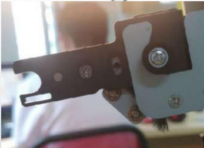
**Solution:** Wrench the Ribbon Led bracket to the normal angle, re-roll the broke ribbon in good condition
