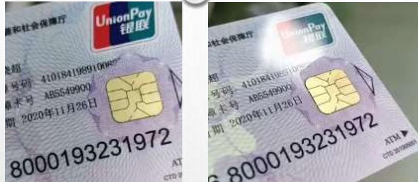
**Cause 2:** There is ink on card surface while printing with no lamination, resulting in unclear printing
