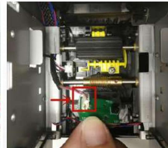
**Cause 3:** Damage of the ADF sensor
