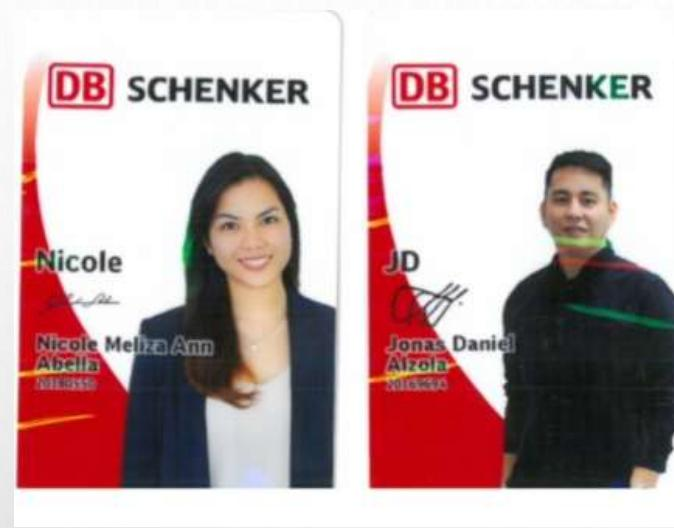
**Solution:** Driver: Print Option - Tools - Ribbon Tension Adjustment - Red End (-)
