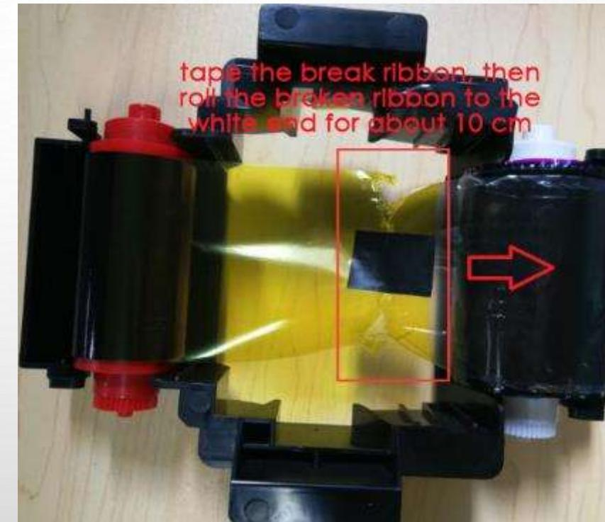
**Note:** If the ribbon breaks often, please refer to the ribbon breakage failure solution
