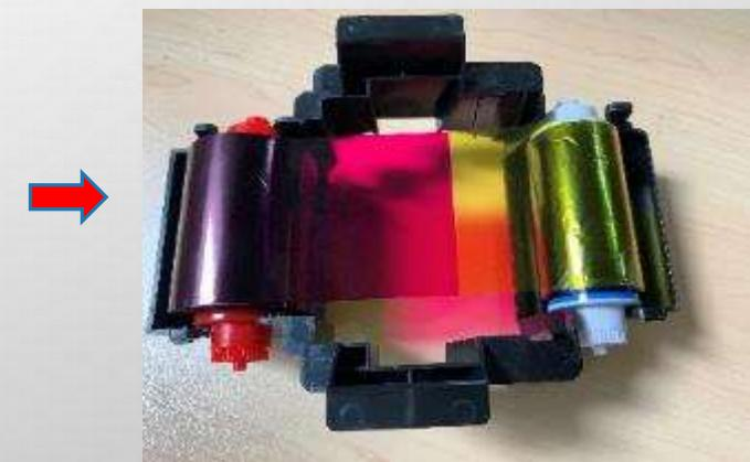
**Note:** The 2 situations for ribbon installed reverse: 1, The color is not installed in correspondence; 2, The color is in correspondence, but the chip direction is wrong
