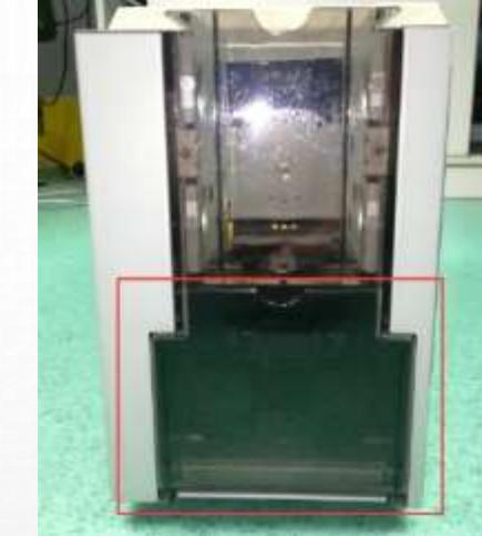
**Cause 2:** Cards in the defective card box are not moved into right place which causing a blocking the sensor
