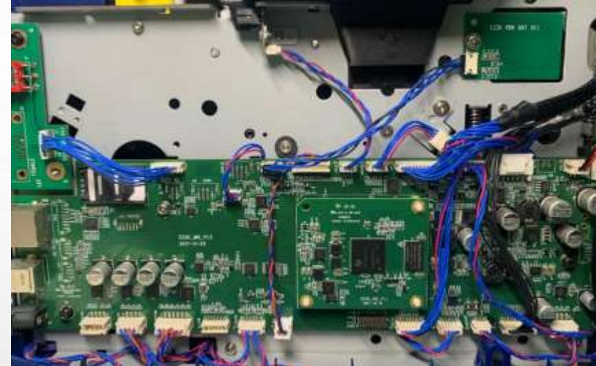
**Cause 6:** The supply and receiving side end of the motor cable abnormal or motor damage (color ribbon)
