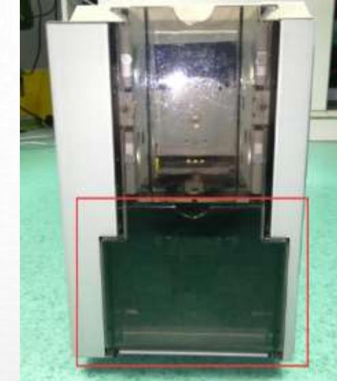
**Cause 2:** The defective card box sensor wiring is loose or sensor is off
