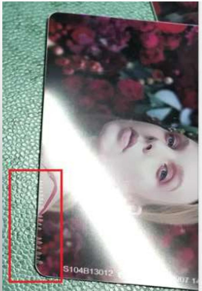
**Solution:** Driver: Print Options - Tools - Ribbon Tension Adjustment
