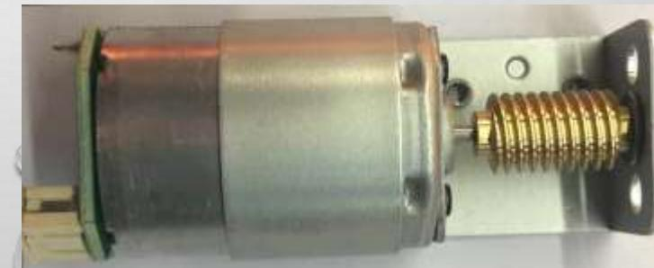
**Cause 3:** The gear of the CAM mechanism is stuck by some other substances.
