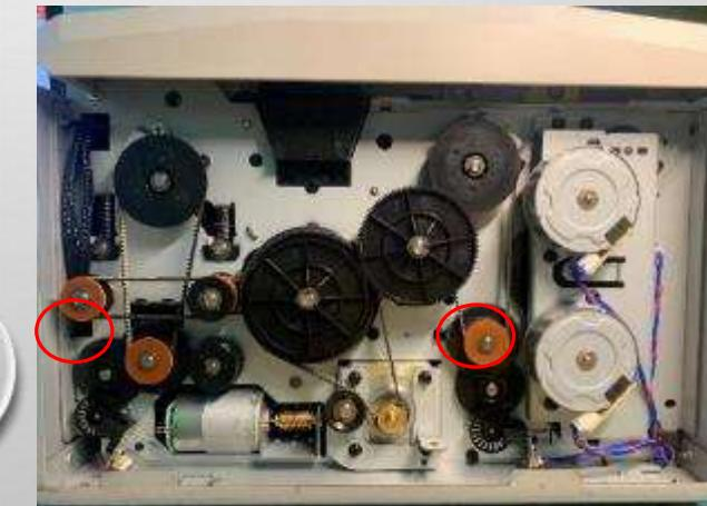
**Causes 3:** the ribbon receiving end of the motor cable abnormal or motor damage (black ribbon)
