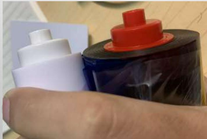
**Cause 5:** The ribbon tension abnormalities causes horizontal lines on image
