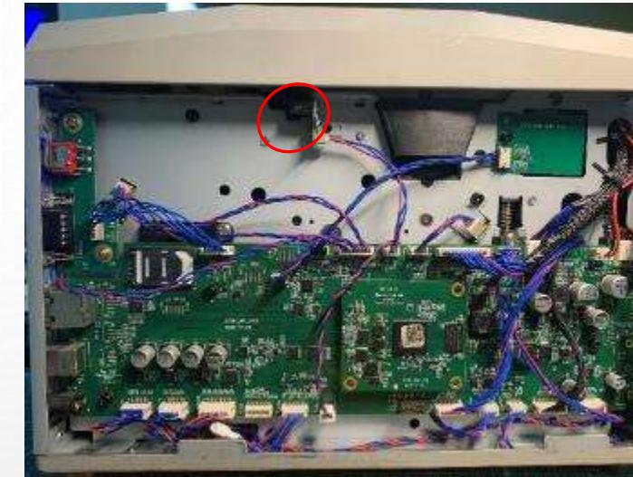
**Cause 2:** The switch sensing mask on the top cover is broken
